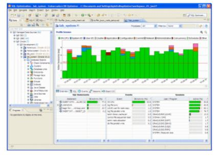
We can see that the CPU load is constantly over the max CPU line. How can we have a bigger CPU load than there are actually CPUs on the machine? Because the demand for CPU is higher than the CPU available on the machine. In the image above there are 2 CPUs on the machine but an average of three users think they are on the CPU, which means that on average one user is not really on the CPU but ready to run on the CPU and waiting for the CPU.
