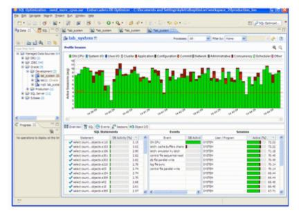
If we look in the bottom left, there is no SQL that takes up a significant amount of load, there is no outlier SQL that we could tune and gain back a lot of wasted CPU. We'd have to tune many SQL and make improvements on most of them to gain back enough CPU to get our load down below the max CPU line. In this case, adding CPUs to the machine might be the easiest and most cost effective solution.
