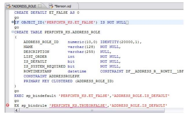
The editor window automatically inserts collapsible nodes in the appropriate lines of code for organizational purposes. This enables you to expand and collapse statements, as needed, while developing code in particularly large or complicated files.
