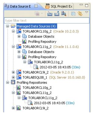
When you next choose to profile a data source, using the **Profile As > Profiling Configurations** option, you can specify the profile repository in which you want to save the profiling session data. You can also access the Profile Repository Preferences from this dialog.
