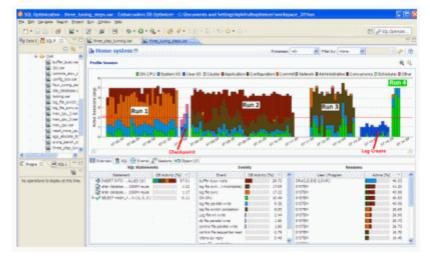
In the above DB Optimizer screen, the same workload was run 4 times. We can see that the time (width of the load) reduced, and the percent of activity on CPU increased. Runs:
