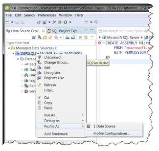
The Data Source Explorer tree provides a list of databases, and enables you to launch Optimizer features, such as SQL Profiler, via the context menu. All objects listed in Data Source Explorer are sorted by data source name. Additionally, you can view the underlying SQL code for an individual database object.
