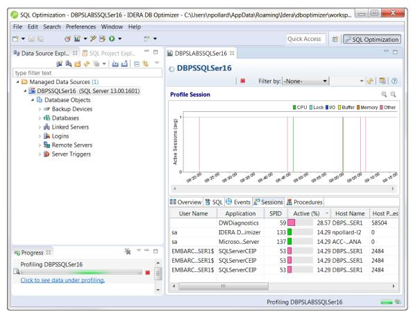
The Workbench provides an environment to build profiling sessions and tune query statements. The **Workbench Space** is composed of views, editors, and the menu bar and command toolbar. Views and editors enable you to perform DB Optimizer functions and work tasks, as well as manage resources.
